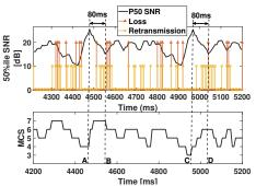
Figure 6: Channel, 50%ile SNR, re-transmissions, Losses and MCS Figure 7: Rate adaptation is unable to keep up with rapid channel changes causing a cluster of losses.
